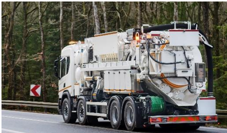
Sewer cleaning equipment
