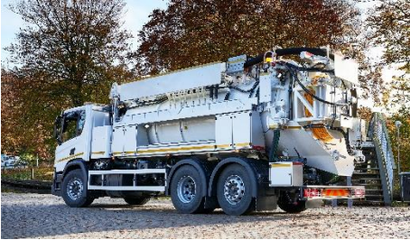
Sewer cleaning equipment
