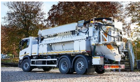
Sewer cleaning equipment
