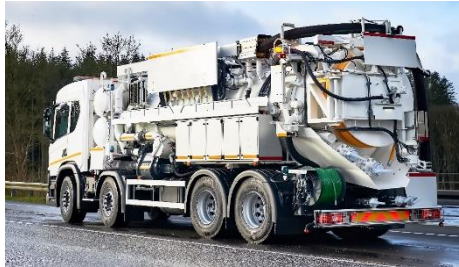
Sewer cleaning equipment
